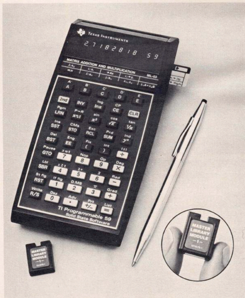
The Texas Instruments TI-59 computer, shown here with one of its plug-in modules. The TI-58, at about half the price, lacks only the capability to handle magnetic chips as well as modules. But the Marine Navigation module, described in the accompanying article, contains more than two dozen programs covering just about any navigational situation
